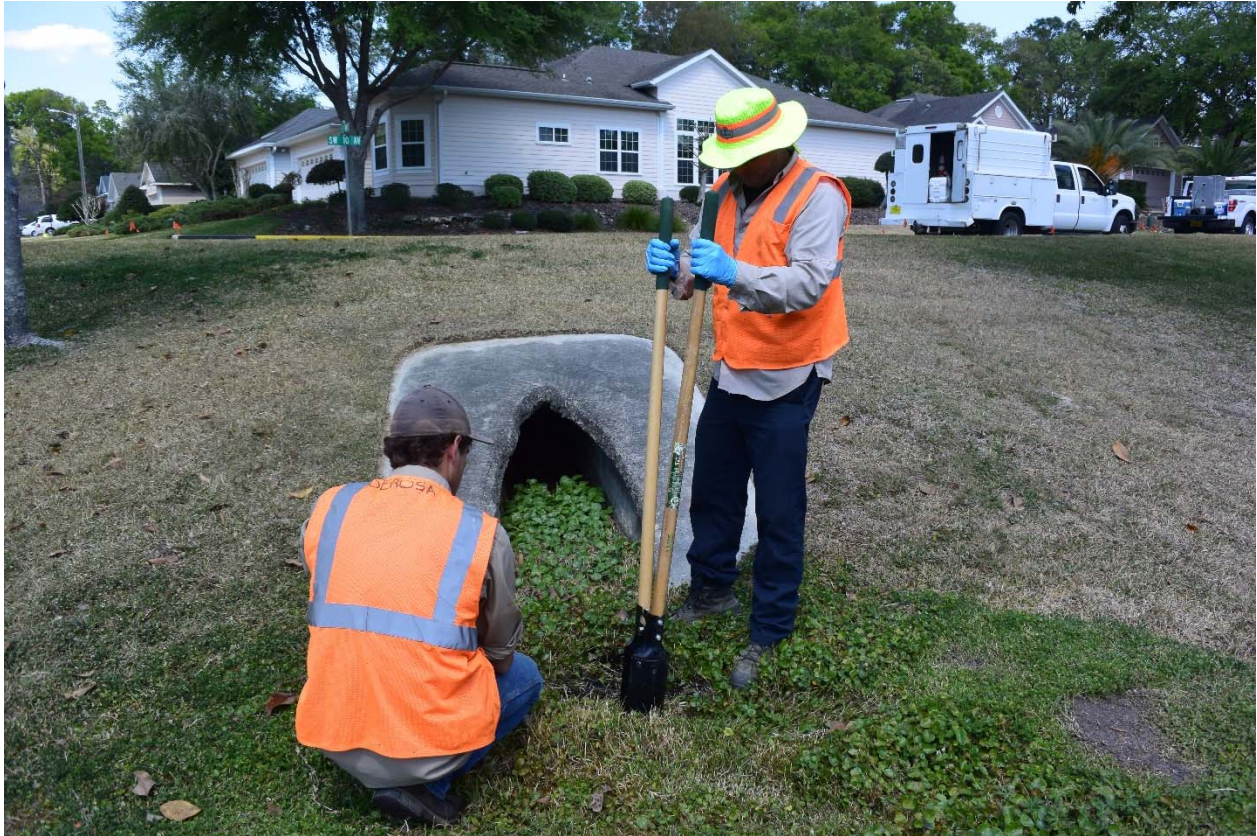
Figure 7 Example of collecting PM samples from best practice management (BMP).
