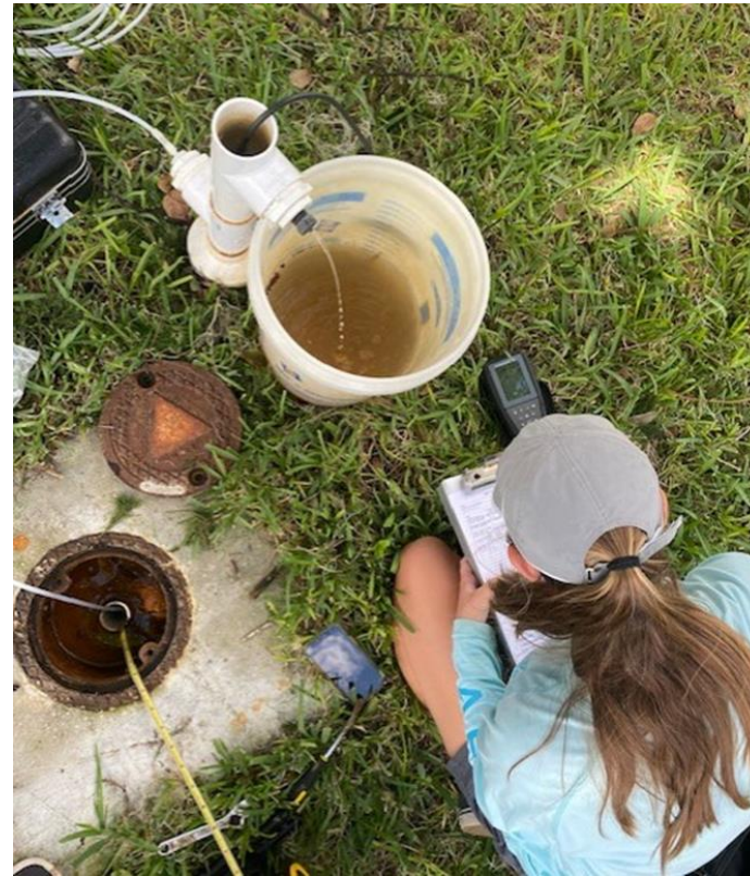
Sampling of a groundwater well
