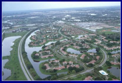
Wet Detention Ponds Can Be Constructed as Amenities
