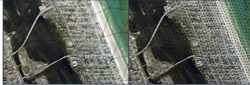
Figure 2 The coarse resolution (100m – 500m) of the HSOFS mesh (left) is to be refined to a resolution of 30m using vertical-feature delineation and RTK-GNSS corrected DEM elevation input.
